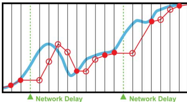
Attempted Solution Increase Profile Generation Cycle Time, but network or backplane delays cause loss of system synchronization resulting in profile execution delays.
