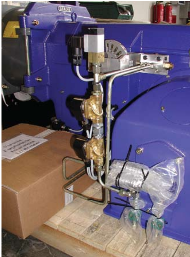
Saacke Eurotherm burner ready for shipping. The couplings are packed to prevent contamination.
