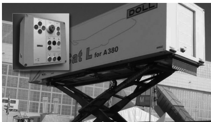
E-Stops can be mounted on a console or on a wireless pendant.
