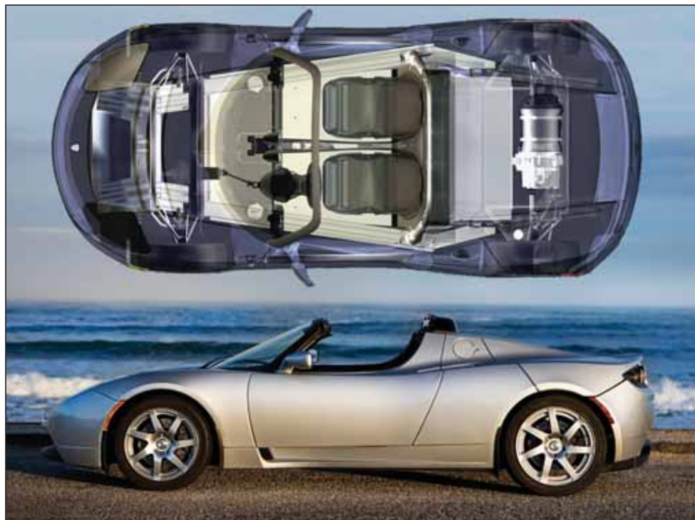
A proprietary 248 hp ac electric motor spins up to 13,000 rpm and weighs less than 52 kg. The battery pack is guaranteed for 160,000 km.
