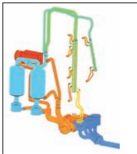
Figure 1: Contours of static pressure on the surfaces of the ozone collection subsystem, one of three that were simulated.
