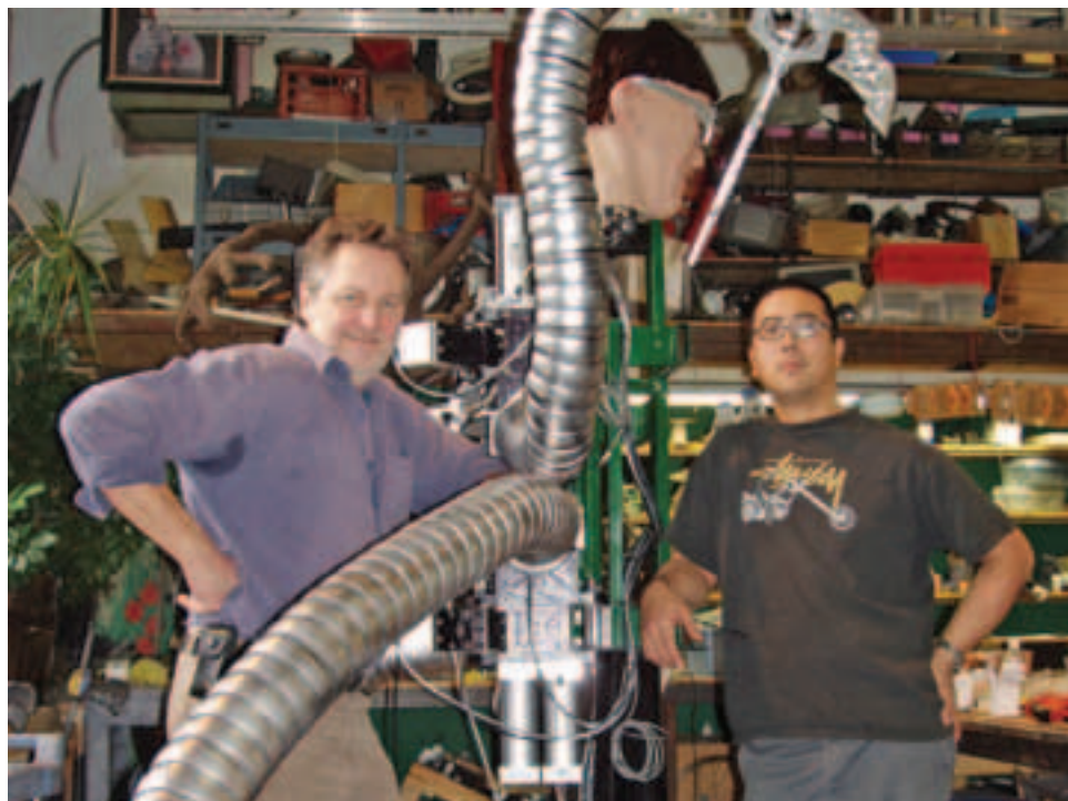
Doc Oc in the shop: Walter Klassen (left) and Taku Dazai pose with the exhibit prior to dressing. Festo CPE14 manifolded valves are used to control head and arm movements.
