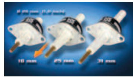
Haydon Switch & Instrument has announced metric strokes of 18, 25 and 31 mm are available on its Z26000 captive linear actuators. The extended travel offerings are available in a wide variety of resolutions ranging from 0.0127 to 0.1016 mm per step and move loads up to 4.5 kg.
