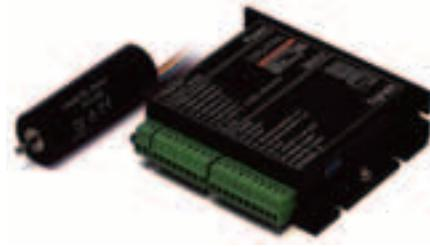
The DECV 50/5 from Maxon is a digital velocity controller designed for controlling brushless motors up to 250 W equipped with Hall sensors. The controller has a speed range of 1000 to 60,000 rpm for 2-pole motors. Requiring a supply voltage of 12 to 50 Vdc, the controller can deliver 95% of the supply voltage to the motor at 5 A continuous current or 10 A peak current. Velocity and torque can be controlled via a 0 to 5 V signal or via external potentiometers.
