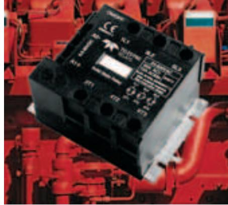
Teledyne Relays has introduced a three-phase induction motor reverser that can be used to turn on an industrial motor in either direction safely. The solid-state series EMCRT is designed to control and invert the direction of a three-phase motor with two of the three legs. The maximum current is 50 A rms (75 A on request). The motor reversers can be mounted on a DIN
