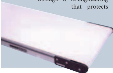
the bearings. Bearings on the conveyors are now installed into a redesigned blind housing hole instead of a through hole. Other features of the series include: instant belt tensioning; V-guide bed plate and belt for positive belt tracking; no special tools required; load capacity up to 80 lb; belt speeds up to 276 fpm; belt widths between 1.75 and 24 in.; and, conveyor lengths between 18 in. and 18 ft.
